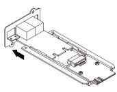
3. Remove the screw holding the RMCARD305 front panel to the card.
