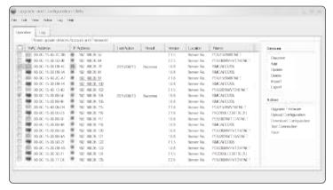
Figure 8. Firmware upgrade success in the main window
