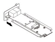
4. Use the two tray screws to secure the card to the adapter.
